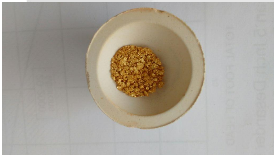
Figure 10: Gold collected from the Screen Fire Assay process is collected in a small crucible
