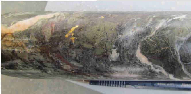
Figure 3: Gold in core from hole QD-44, Querosene prospect. This interval from ~148m depth, yielded ~1,992 g/t gold and is logged as hydrothermalite.
