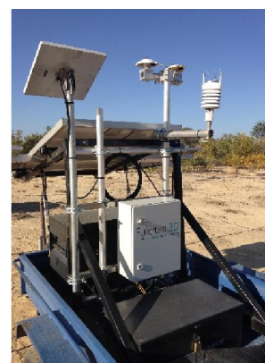
Solar monitoring station at Kidston
