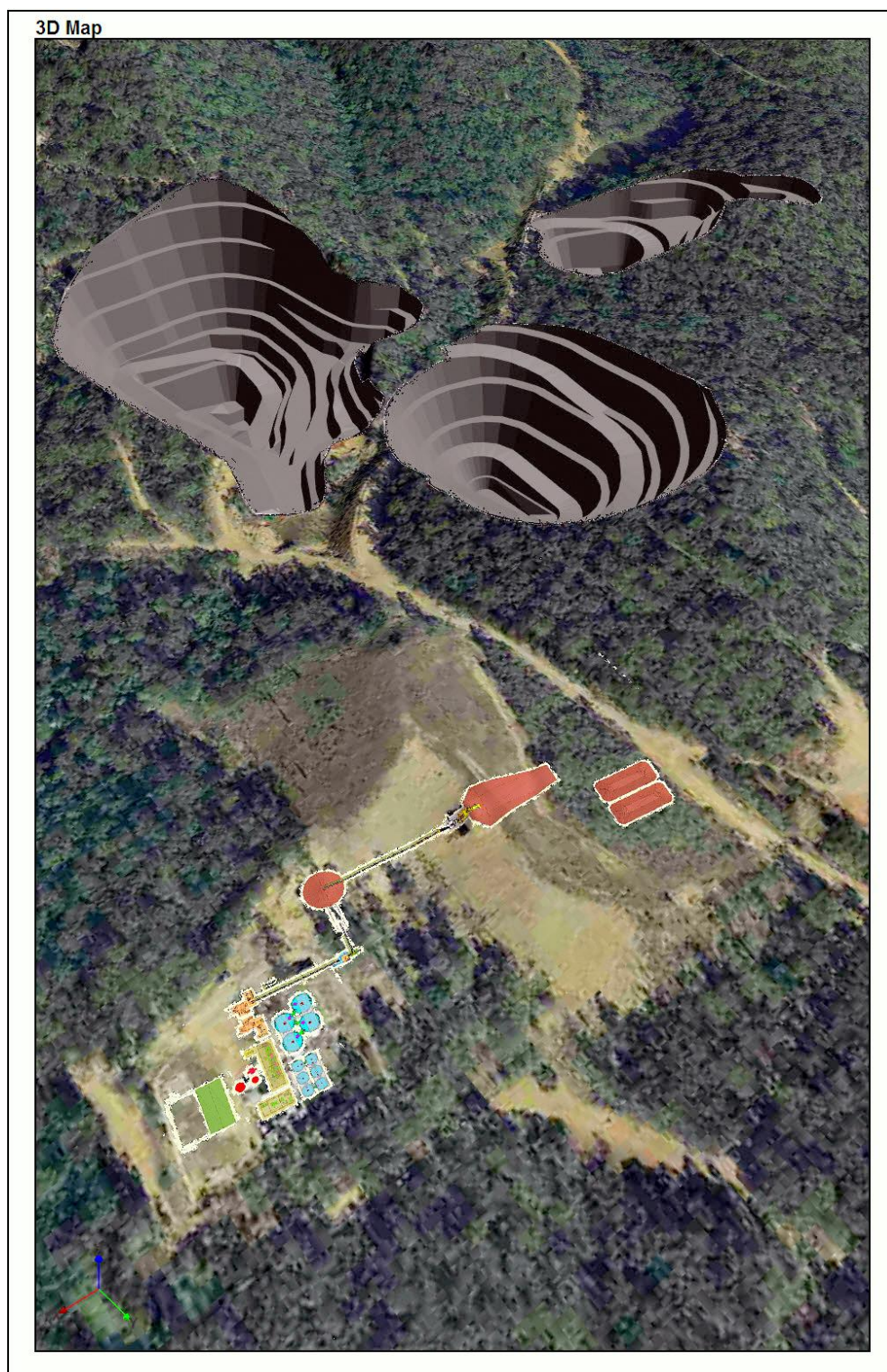
Figure 1: Aerial view towards the south-west looking down on the preliminary pit designs for the Strauss and Kylo gold deposits, and showing their close proximity to the processing plant layout which will utilise the existing foundations and haul roads.
