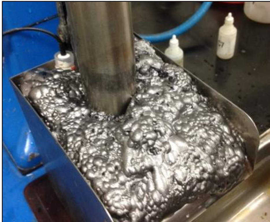
Image: GS03 Weathered Composite Rougher Flotation without Collector
