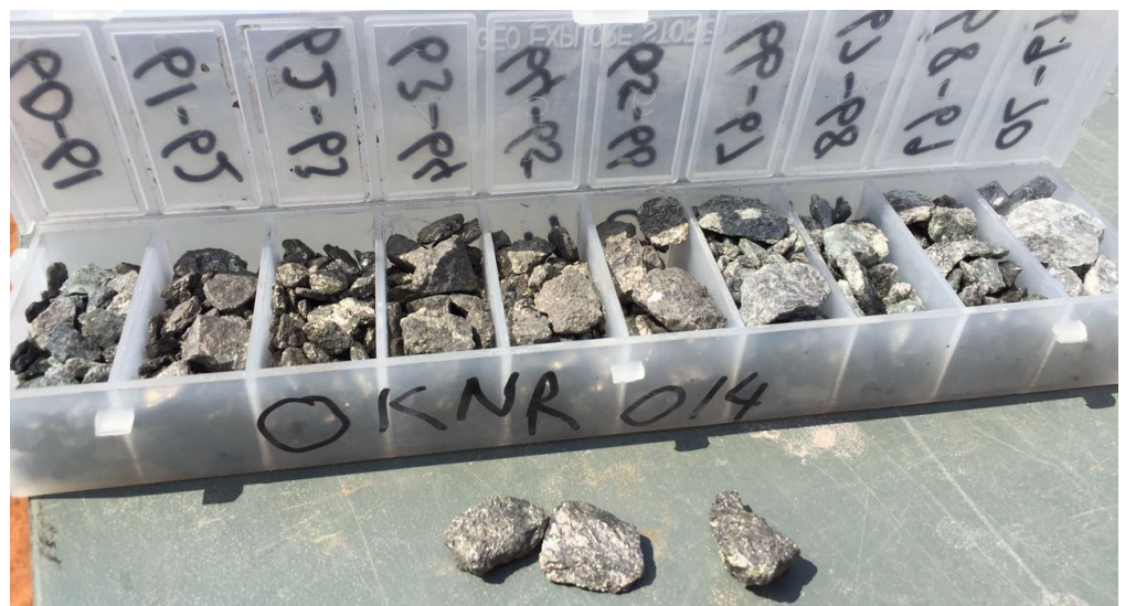
Figure 1: Massive sulphides in OKNR014 which returned 7m at 6.44% Zn and 0.43% Cu from 60m. Note each divider shows chips from a 1m interval.
