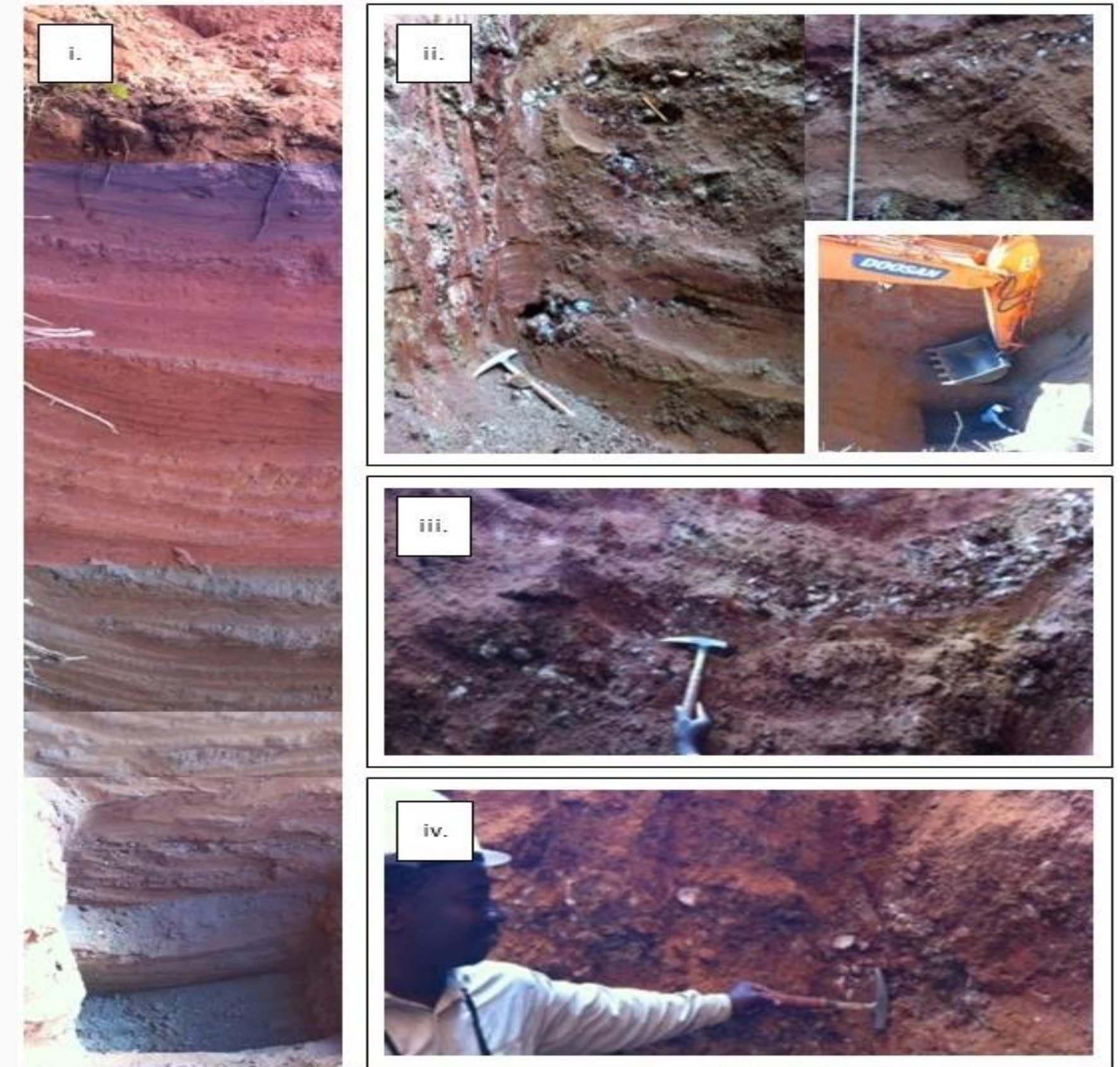
Stratigraphy of Secondary Ruby Deposit on License 4143L; Images of EXPIT 021; (i.) Composite profile showing the change in colouration and material; (ii.) NW Face, showing gravel from 7.3 to 7.7m, with larger clasts; (iii.) SE face showing dip of gravel to north; (iv.) NE face showing approximately 40cm layer of gravel.
