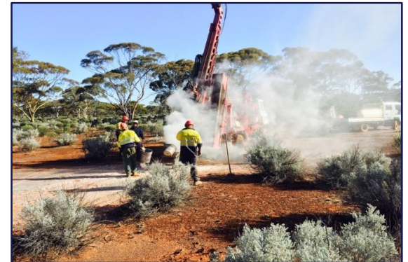
RAB Drilling at Torian's Zuleika JV Project.
