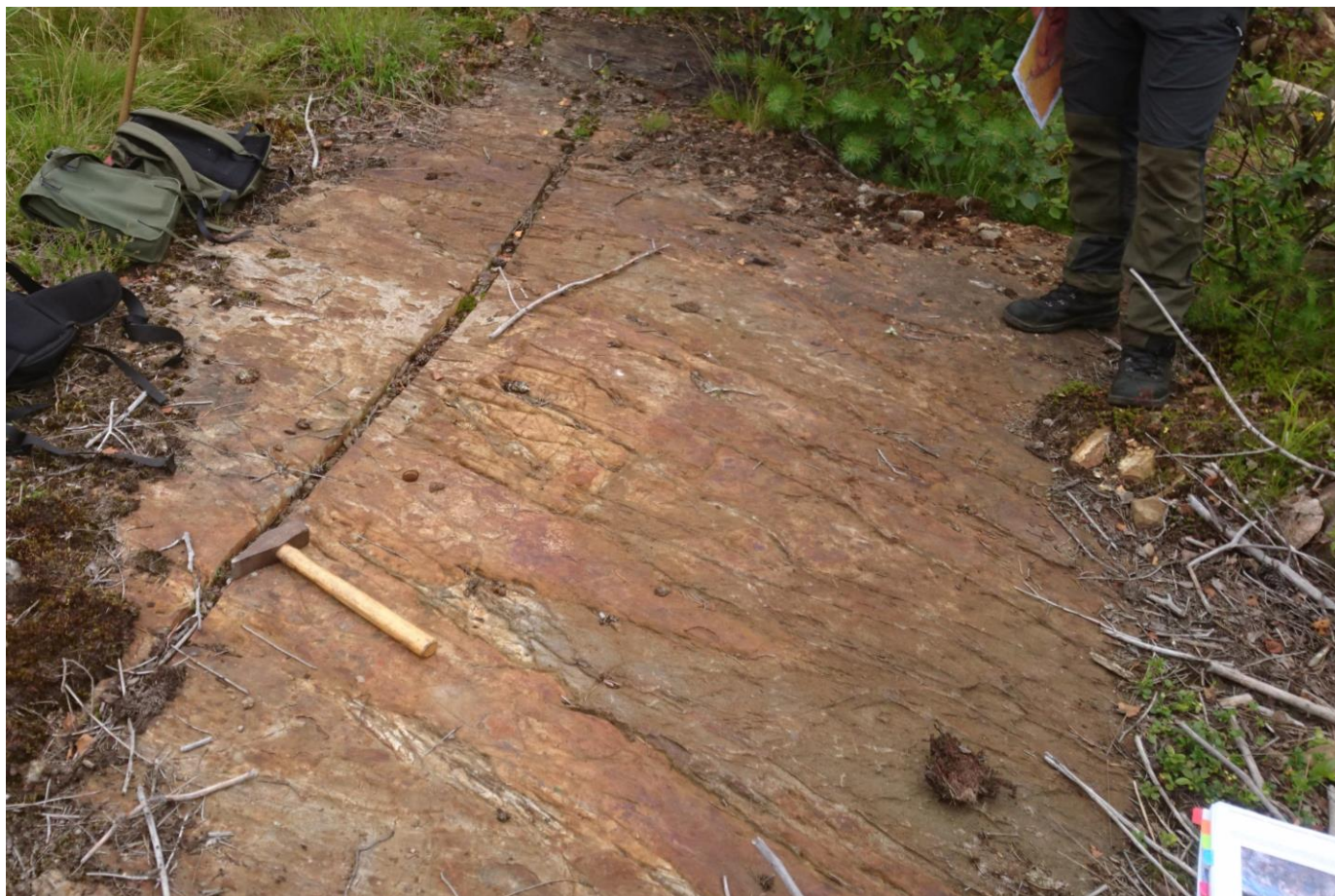
Figure 3: Photograph showing quartz veined and sulphidic outcrop at the Satulinmäki gold prospect and the 2003 GTK 5m channel sample which returned assay results of between 1.9 g/t and 8.5 g/t Au. Drill hole R391 was drilled below this outcrop and returned values of 25.0m @ 3.17g/t Au including 3.0m @ 9.3g/t Au, and 4.0m @ 10.3g/t Au.
