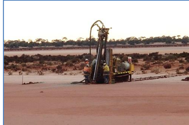
Track-mounted Aircore Rig
