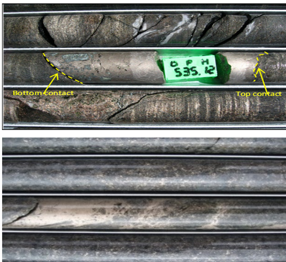
Figure 9: Photos of historical drill core from the Jacomynspan Project, including massive sulphide zones grading up to 4.2% Nickel.
