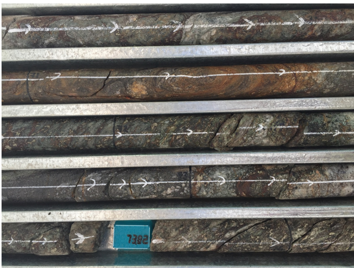
Figure 4: Highly mineralised core intersected in hole OWCD033 between 70 – 74 metres. Pyrite (5%-15%) is partially oxidised to haematite and limonite at this depth. Lithology is structurally complex, folded and sheared. The white line marks orientation reference line.
