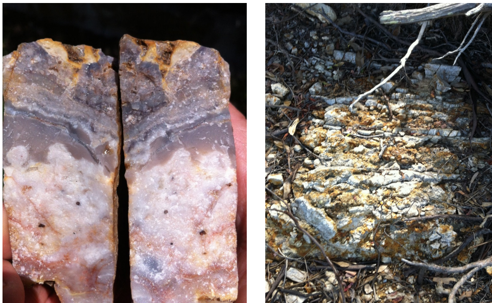
Figure 17: Samples from field mapping showing epithermal vein textures (LHS) and sheeted quartz veins in outcrop (RHS).
