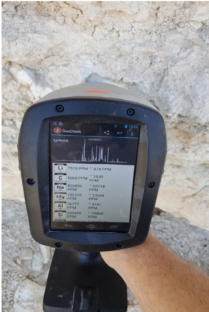
Figure 1: Spot reading of 7,919PPM Lithium (4.2% LCE) at Muddy Mountain
