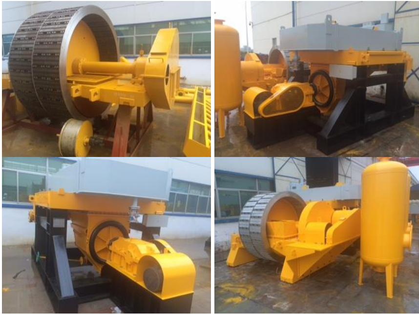
Magnetic separation equipment painted post testing and ready for packing
