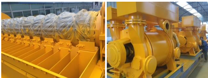
Water filtration equipment painted post testing and ready for packing
