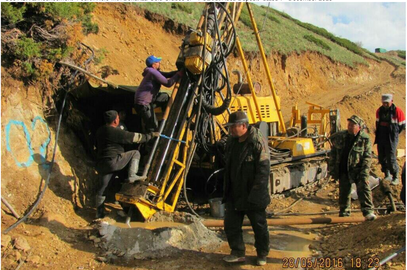
Figure 1: Diamond drill rig and crew starting the 2016 drill program at hole EGZ16-002 which is targeting a mineralised zone 50 metres below a 2015 drill intersection of 3 metres at 41.4 g/t and 1 metre at 58 g/t.
