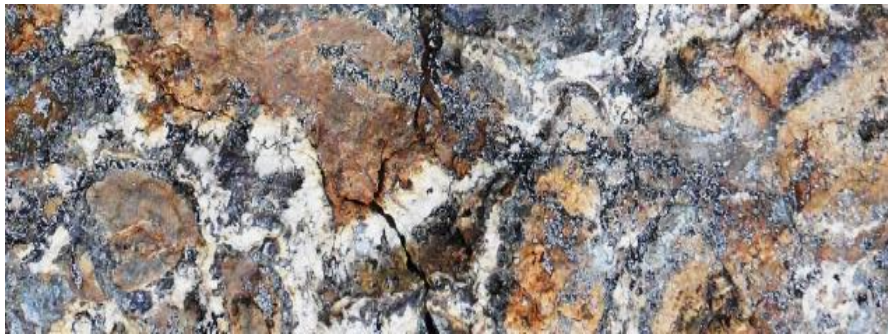
Figure 1: LEFT Brecciated dolomitised limestone with iron oxides and sulphides from a mineralised vein at Riqueza grading 12.45% Zn, 195g/t Ag and 17.41% Pb.
