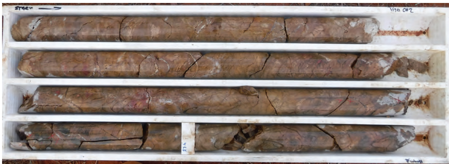
YMD002 CORE – GOLD MINERALISED BRECCIA AT BOX WELL PROSPECT
