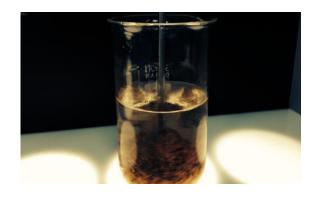
2. Fix & achieve consistency of good flocculation. Inconsistency was caused by changing levels of **clays** in the feed.
