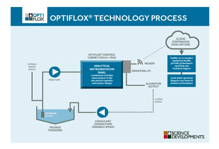
This technology is therefore able to consistently and accurately know when to dose coagulant, define how much coagulant should be dosed and know when to stop coagulant dosing.
