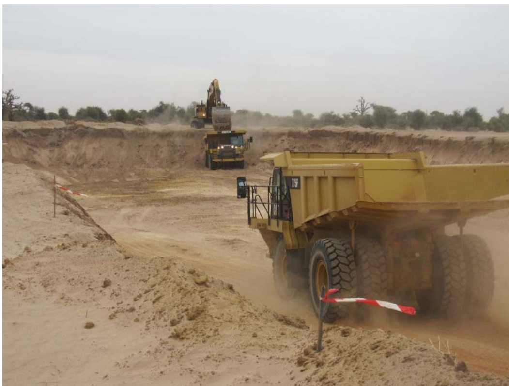
Figure 1: Stage 1 Open pit access ramp establishment in progress
