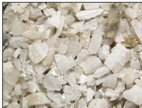
DMS Concentrate 3.35mm SG 3.1 overflow predominately white spodumene, <0.2% mica
