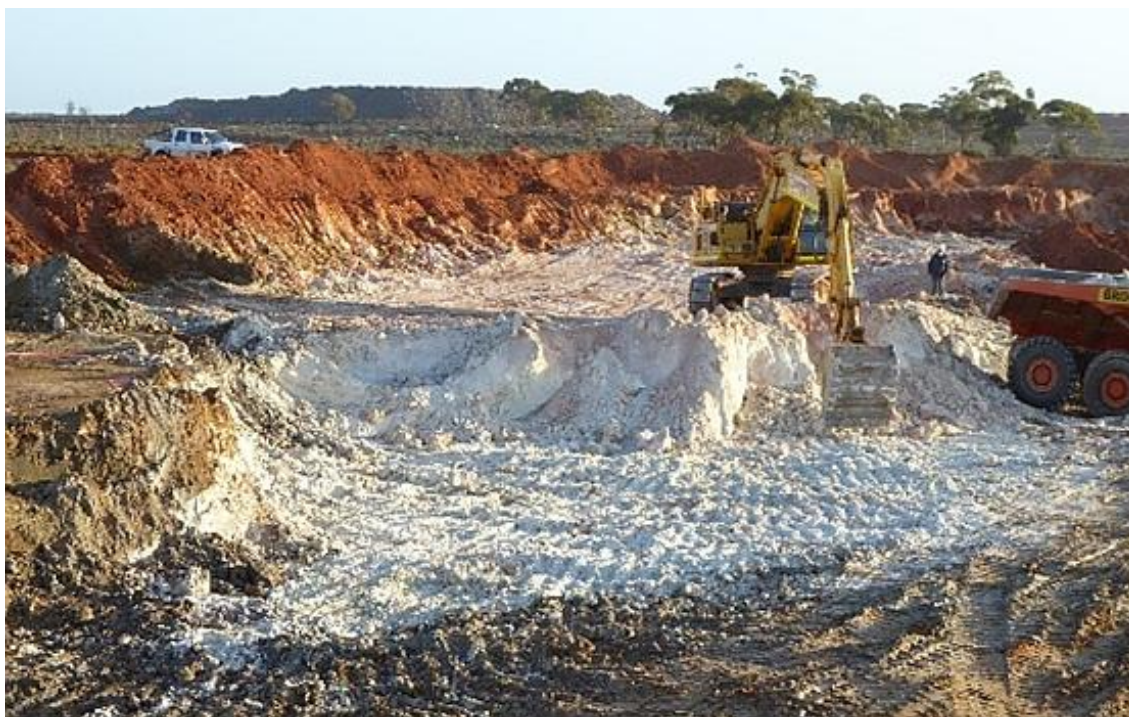
Mining of Weathered Pegmatite, Boreline Extended Pit 2015.
