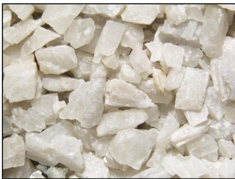
DMS Concentrate 3.35mm SG 3.1 underflow. High levels of white spodumene
