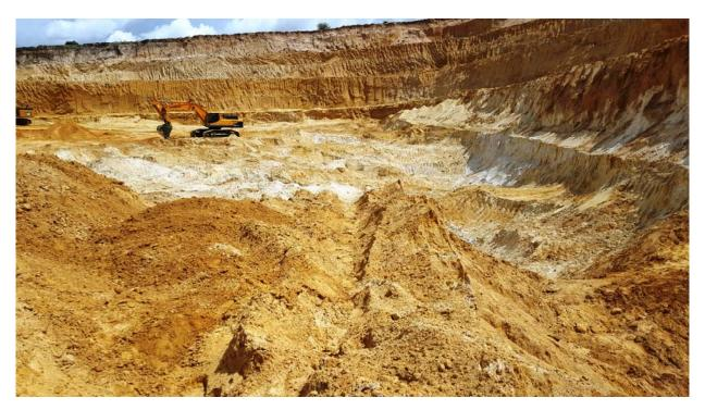
The mineralisation exposed is consistent with the geological model derived from air core and diamond drill logging and sampling and it is expected that primary grade control will be visual.
