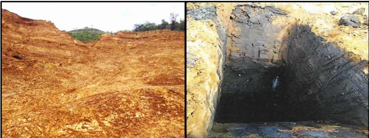
Figure 3. Sandstone Gully. a) Thick tailings exposed in the upper reaches of the southern Sandstone Gully - 0.33m average oxide crust at surface, and b) test pit TP5 showing sulphidic tailings with thin oxide crust, southern Sandstone Gully.
