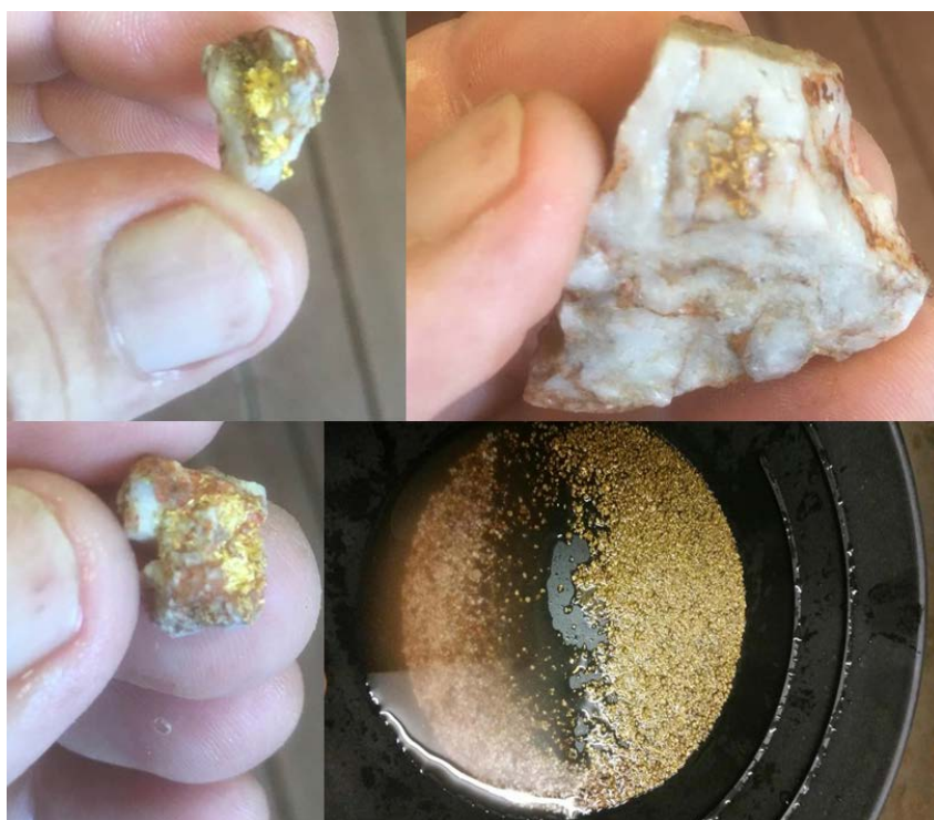
Figure 1: Selection of gold samples discovered by a prospector on drill pads excavated for the drilling program. Bottom right picture shows gold which was produced by crushing quartz vein samples collected from drill pads. There has been insufficient work to determine a Mineral Resource and it is uncertain whether further exploration will result in the determination of a Mineral Resource.
