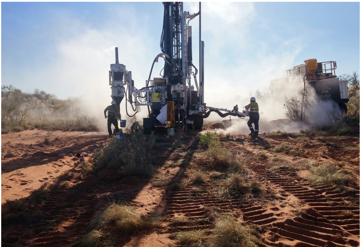
Figure 1 – Aircore drilling rig operating this week at the Obelisk copper-gold anomaly, Great Sandy Project
