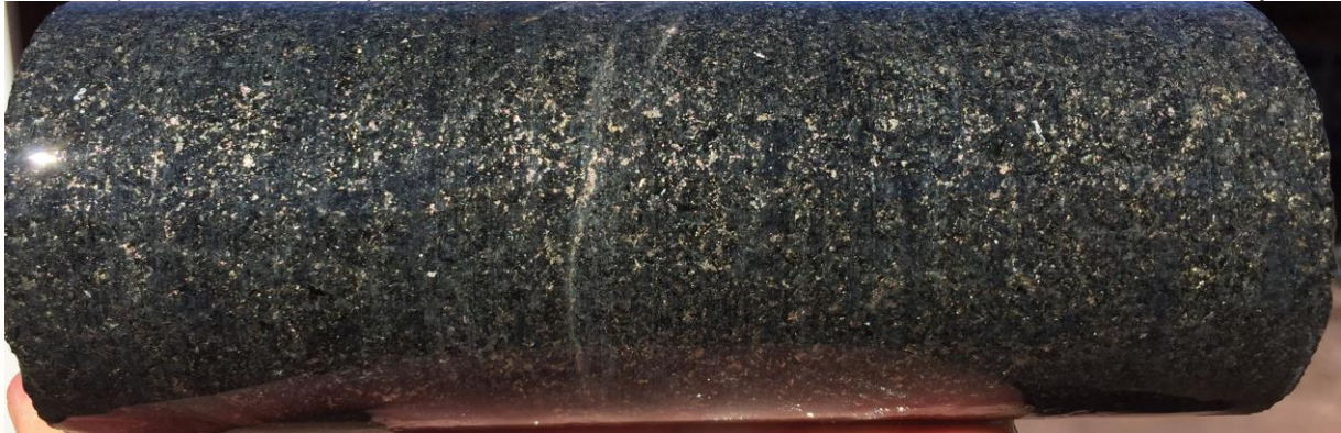
Figure 1 – Disseminated primary Ni-Cu sulphides in hole DMDD001 (56.37-56.53 metres, HQ3 61mm diameter) at the Merlin Prospect. This mineralisation is non-conductive and cannot be detected by TEM.
