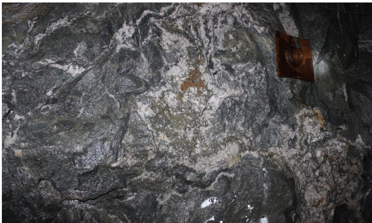
Photograph 7: Gold-bearing pyrite–chalcopyrite–quartz breccia near the western margin of G lode exposed in underground development
