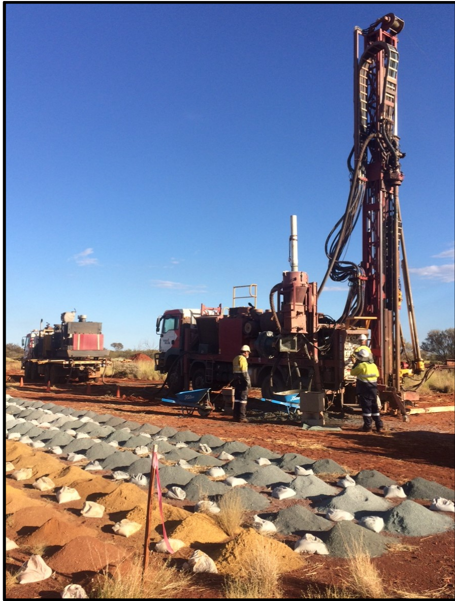
RC drilling rig in operation at the Bibra Gold Deposit, Karlawinda Project (5 th April 2016)
