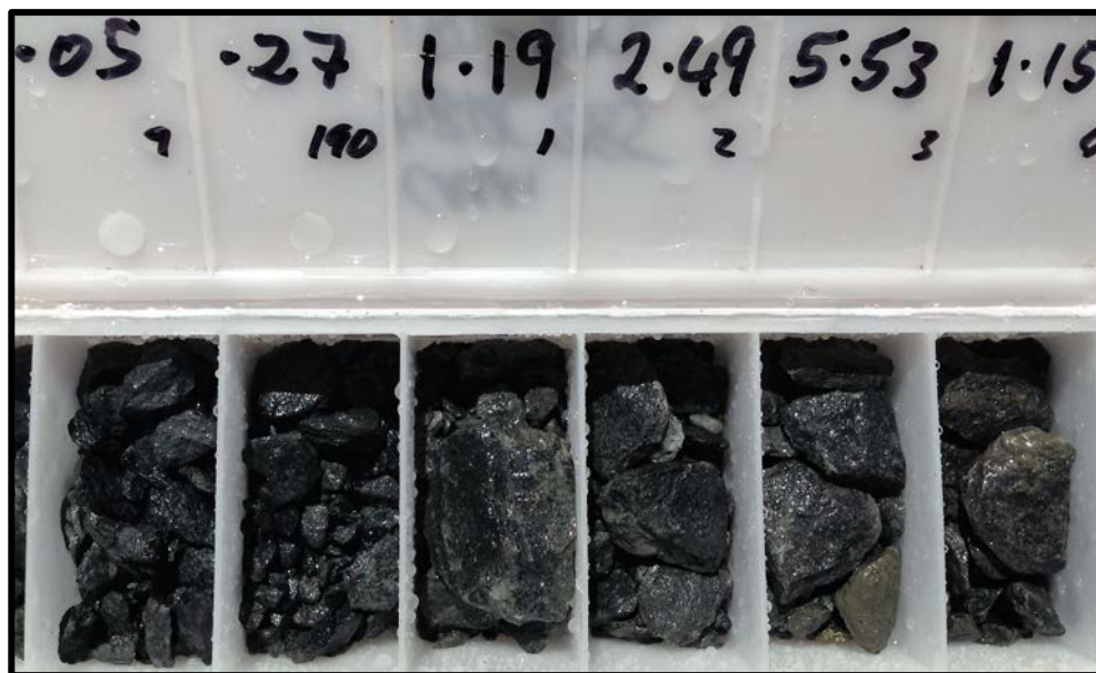
RC drill chips from drillhole KBRC 285, in 1m increments from 189m to 194m downhole (Total intersection 9 metres @ 5.1g/t Au).
