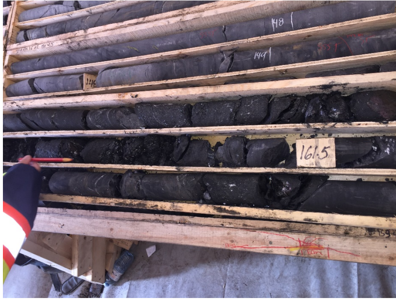
Figure 2: Panorama North core logging operation – coal intersection
