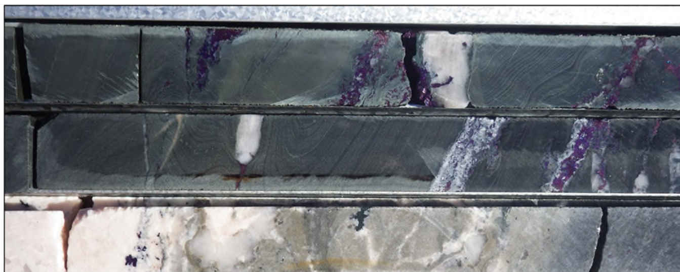
Figure 3: Example of Bornite vein hosted mineralisation in drill core from MO-G-01D (Assays awaited)
