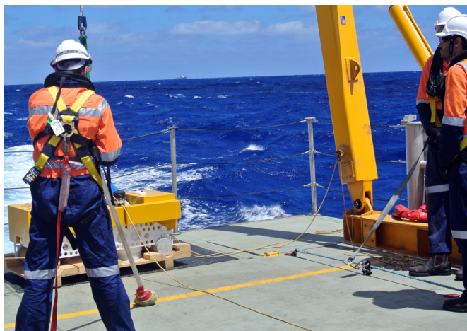
OBS being prepared for deployment as CCG's Viking vision is shooting the BART 3D reflection survey.
