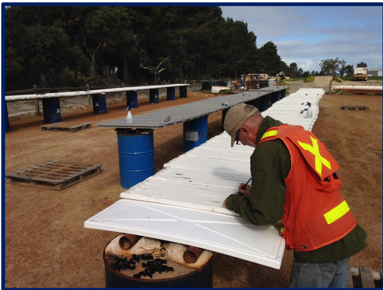
Figure 1: CSA Global nickel sulphide expert Tony Donaghy re-logging MRDD016 core.
