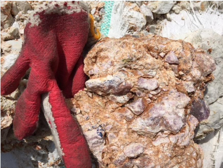
Figure 5: Lithium mineralised breccia sample, Boam Mine (not an asset of the company)
