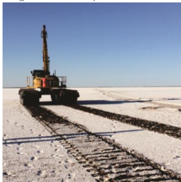
Figures 5&6 – Amphibious Excavator Operating on LD
