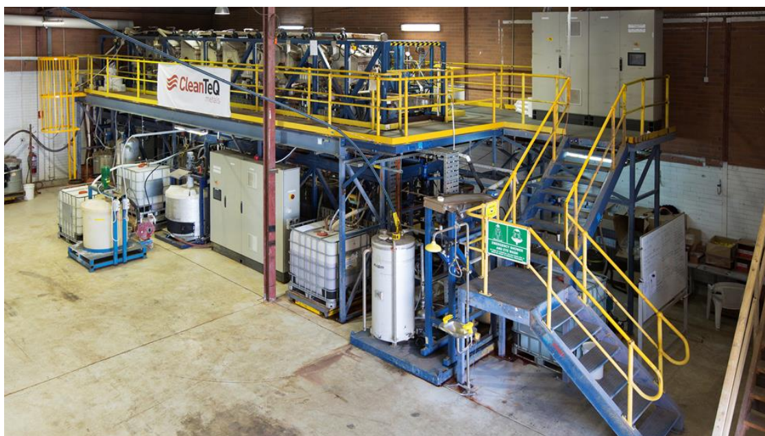
Figure 5: Clean TeQ's proprietary Resin-In-Pulp (RIP) process demonstration plant, which is to be used for production of \text{NiSO}_4 and \text{CoSO}_4 samples for customer testing
