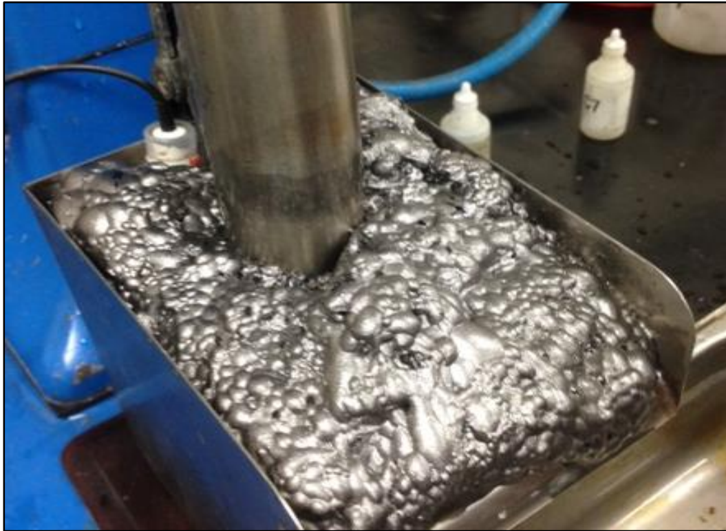
Image: GS03 Weathered Composite Rougher Flotation without Collector; Chemical free production from MTA's graphite
