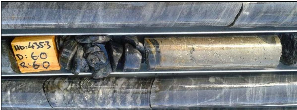
Figure 4: Narrow stringer of remobilised nickel sulphide grading 10.2% Ni in PLJD0001.
