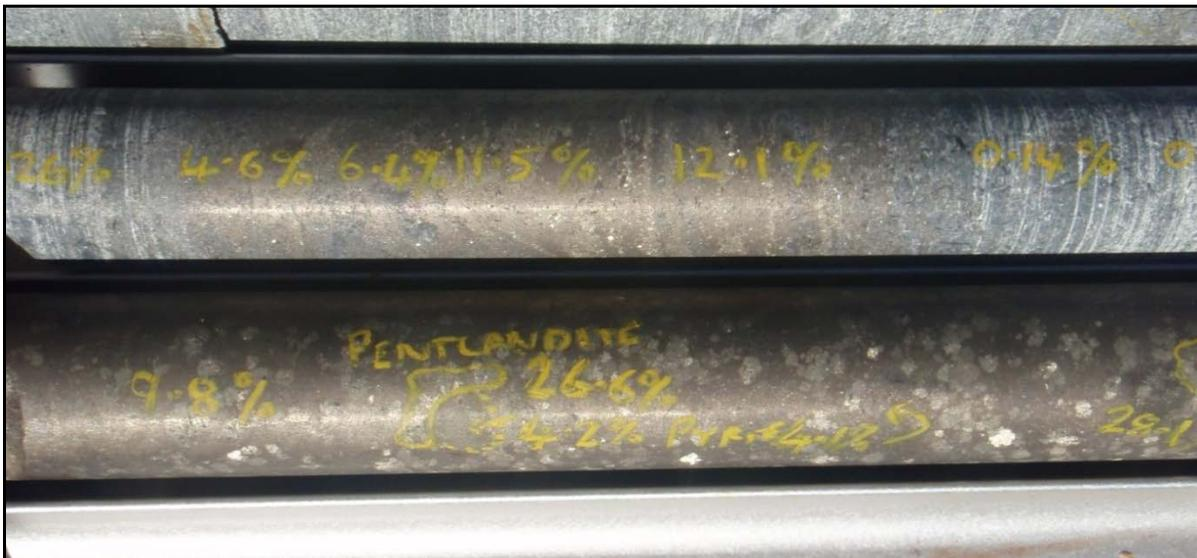
Figure 5: High grade massive nickel sulphide (pentlandite) intersected in PLJD0002 (439.6-440.8m depth) 350m north of Emily Ann mine with localised in-field Niton pXRF Ni% readings recorded on the core.
