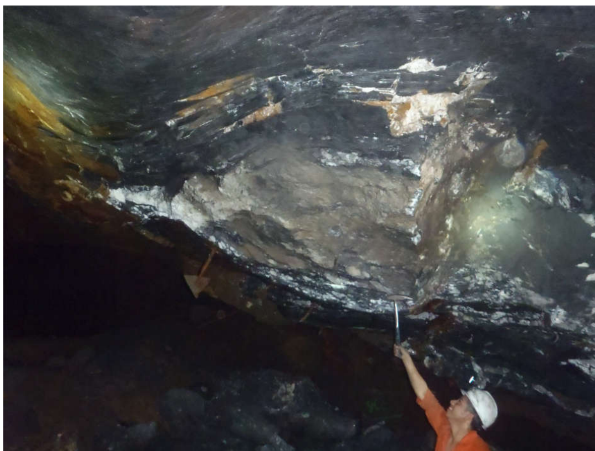
Figure 4. Boudin of marble and sulphide within the hangingwall shales at the 8.1 drill drive turn-out
