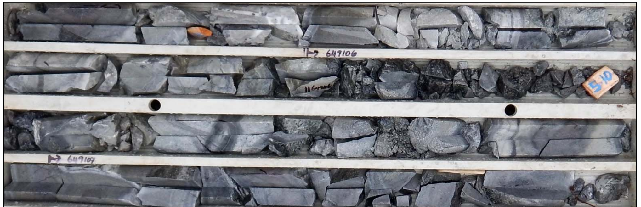
Hole EZU001 from surface (in upper left) to 2.10m. Native gold was located on core saw cut at 0.70m (red ellipse above). Core tray is 1.0m long internally. Photography is currently incomplete for Hole EZU001 from approx. 2.1m to 3.1m.
