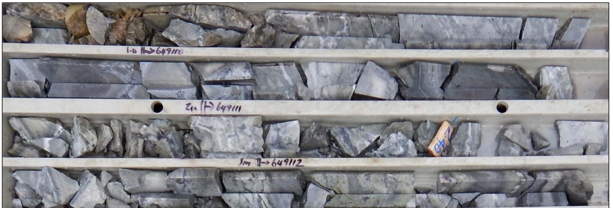
Hole EZU001 from surface (in upper left) to 2.10m. Native gold was located on core saw cut at 0.70m (red ellipse above). Core tray is 1.0m long internally. Photography is currently incomplete for Hole EZU001 from approx. 2.1m to 3.1m.
