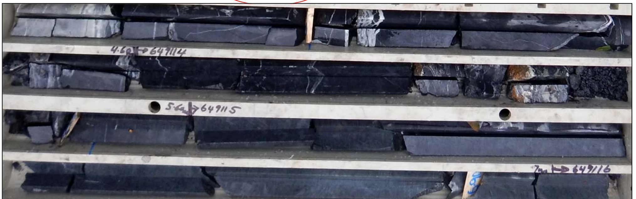
Hole EZU002 from surface (in upper left) to 7.1m. Red ellipses at 1.15m and 3.00m show the core in which native gold was located and photographed. Hole EZU002 has a slight 3D effect as the quarter core is sitting on top of the half core (i.e. the front quarter core has been sampled).
