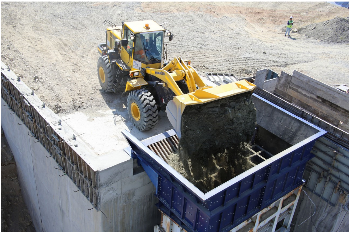
The first bucket of stockpiled ore being tipped into the headfeed bin and primary crusher
