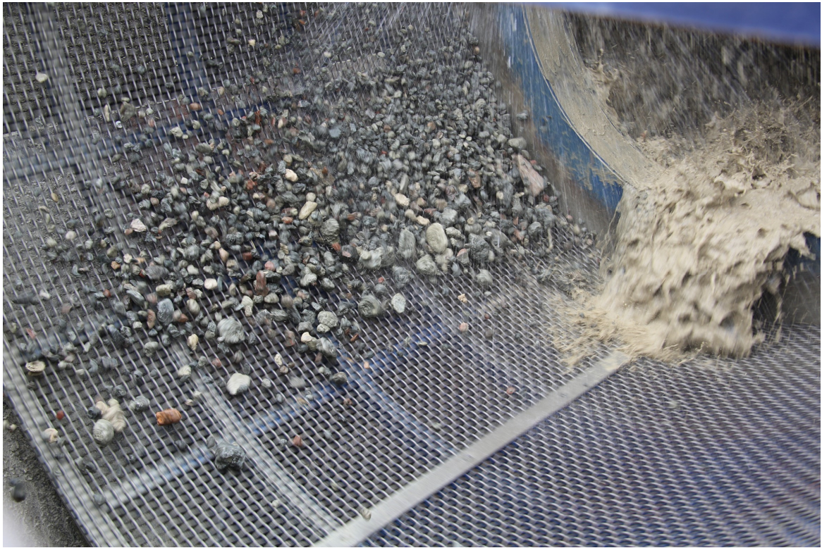
First ore being sorted in the primary scrubber trommel screen
