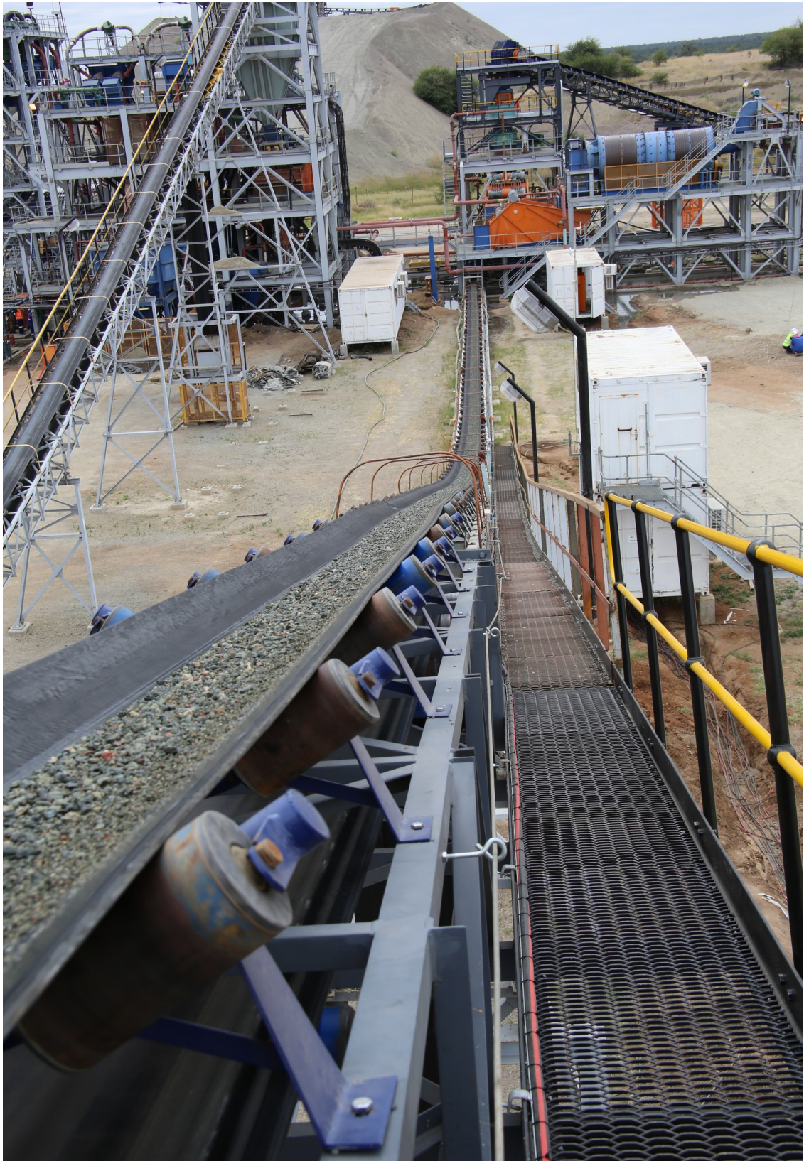
Ore on its way from the secondary scrubber to the 400 ton surge bin, feeding the DMS
