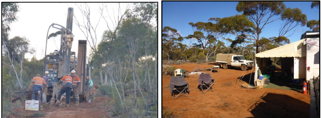
Figure 2 – Aircore drilling rig (left) and exploration camp (right), Western Margin Prospect
