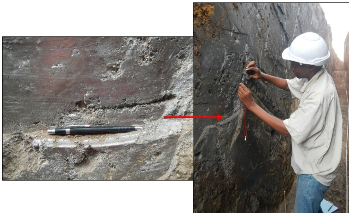
Figure 2: High grade weathered graphite zone – 9.3m @ 22.6% TGC including 4m @ 25.2% TGC and 2.2m @ 38.5 % TGC - in trench LJTR002 from 24m to 33.3m.
