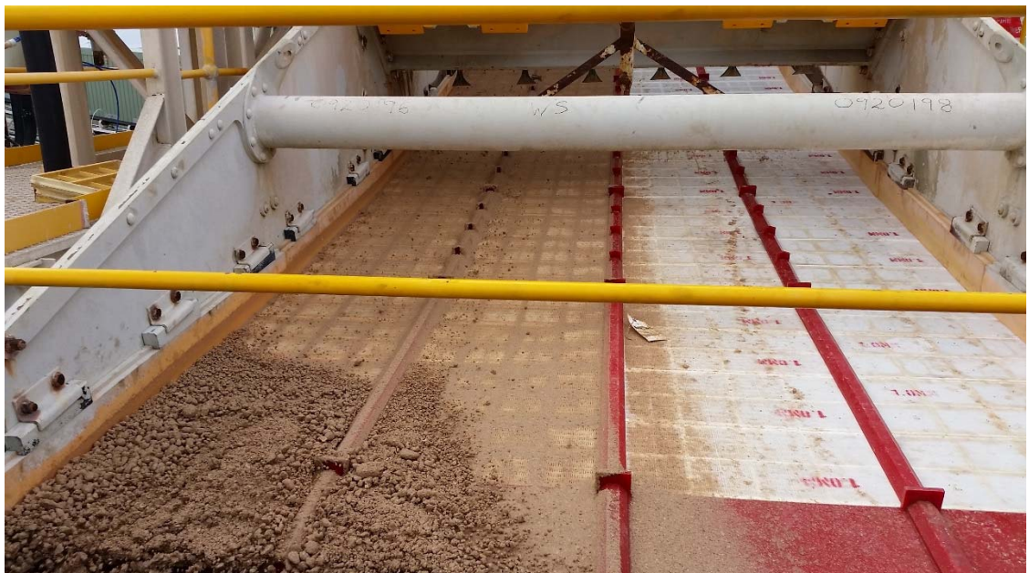
Figure 2 Feed preparation circuit primary screen
