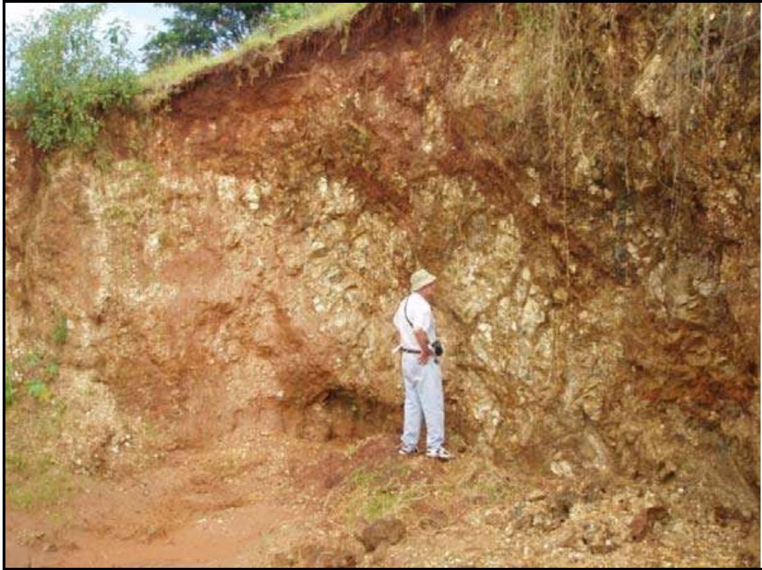
Photo 2: Very coarse grained vermiculite zone - NW wall of the Namakera open pit on ML4651.
