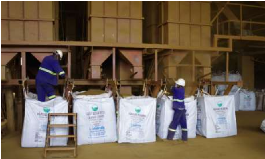
Photo 14: Final Screening and Bagging of the Product Within the Plant Located on ML4651
