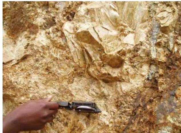
Fresh, coarse grained vermiculite exposed in the open pit on Mining License ML 4651
