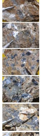
**Photo 1:** Mineralised vein sample. Fine matrix of sulphides (<u>sphalerite</u> – a zinc sulphide and <u>galena</u> – a lead sulphide) with Fe-oxides (red-brown) and barite (creamy white). Barite is a common gangue mineral in Zn-Ag-Pb ores in several types of deposits, especially replacement deposits, such as that at Humaspunco. Fe-oxides have developed as weathering products of sulphides and carbonates. **17.03% Zn**, **293g/t Ag**, **13.07% Pb**.
