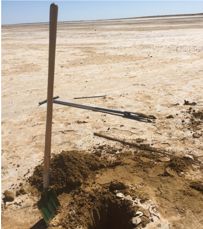
Figure 2: Lake Gregory Pit 1 excavated and hand-augered to 0.94m. Standing water level - 0.69m.
