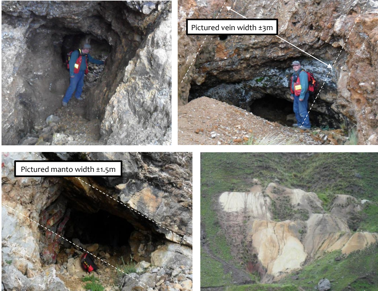
Figure 3: Mining workings within the project area TOP LEFT & RIGHT Mine workings at Santa Rita accessing vein mineralisation. Qtz/carbonate veinlets show the near-vertical main Ag-Pb-Zn mineralised vein. BOTTOM LEFT Working into the mineralised manto, where mineralisation is conformable with the bedding. BOTTOM RIGHT The main Rita Maria mining workings.
