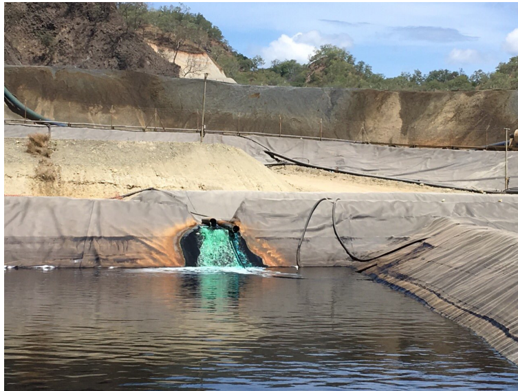
Image 4 – Primary leach solution flowing from the KKV heap leach pads
