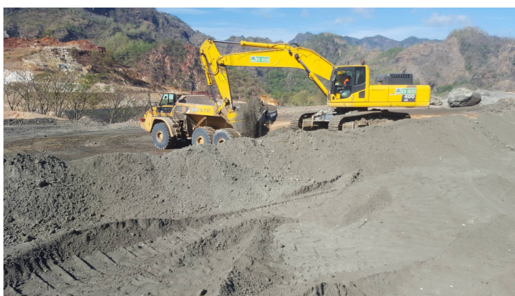
Image 1 – Excavating blasted material in Kali Kuning pit
