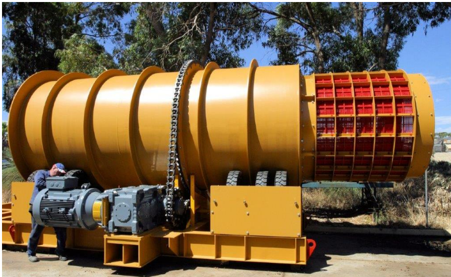
↑ Attrition scrubber of the type that could be used for a saprolite-hosted graphite operation
