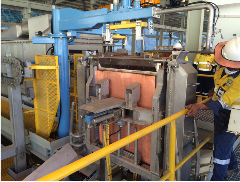
Figure 2: Copper cathode stripping machine at the 25,000 t.p.a. SX-EW plant.
