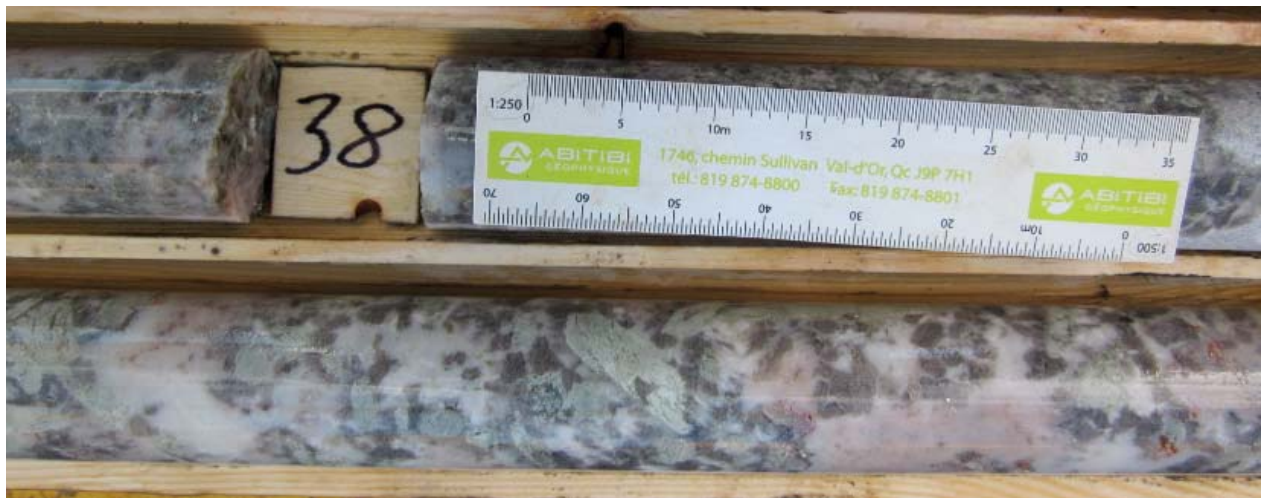
Dempster L61 East Pegmatite. Note light green lithium-bearing spodumene. Spodumene is the main lithium mineral found in pegmatites ( \text{Li}_2\text{O} \cdot \text{Al}_2\text{O}_3 \cdot 4\text{SiO}_2 , theoretical \text{Li}_2\text{O} content of 8.03%). (Drill Hole CL-16-06, around 38 – 39 metres downhole, scale NQ Diamond Core 47.5mm diameter)
