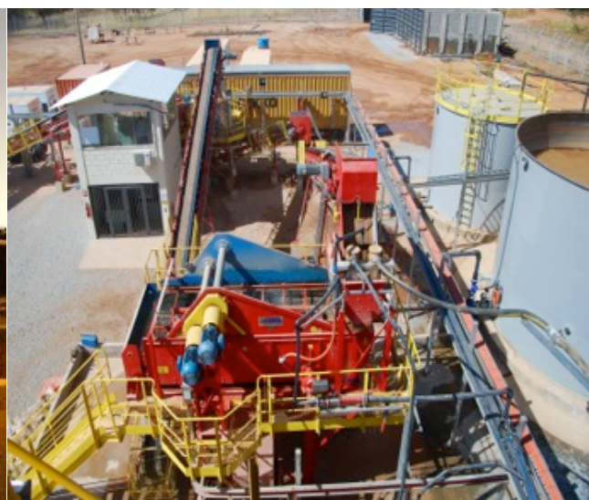
Figure 1. Left: Gravity circuit during night shift. Right: Vibrating screen between the comminution and gravity circuits with oversize material re-circulating back through the comminution circuit.
