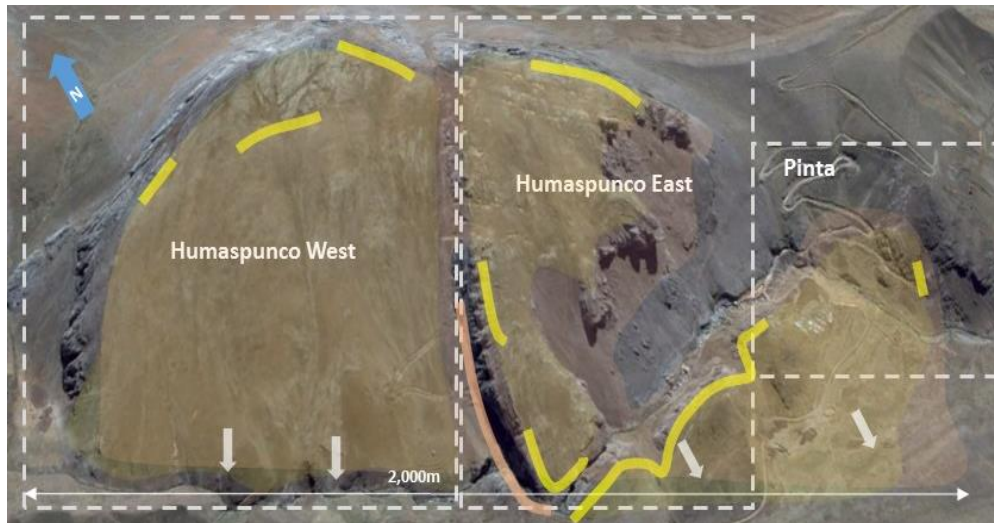
Figure 5 LEFT: Satellite image showing the Humaspunco and Pinto Prospects. The pale yellow shading shows the projected expanse of the upper manto sequence, connecting outcrop occurrences of three manto horizons (thick yellow lines). The pink shading shows the projected expanse of the lower manto sequence.
